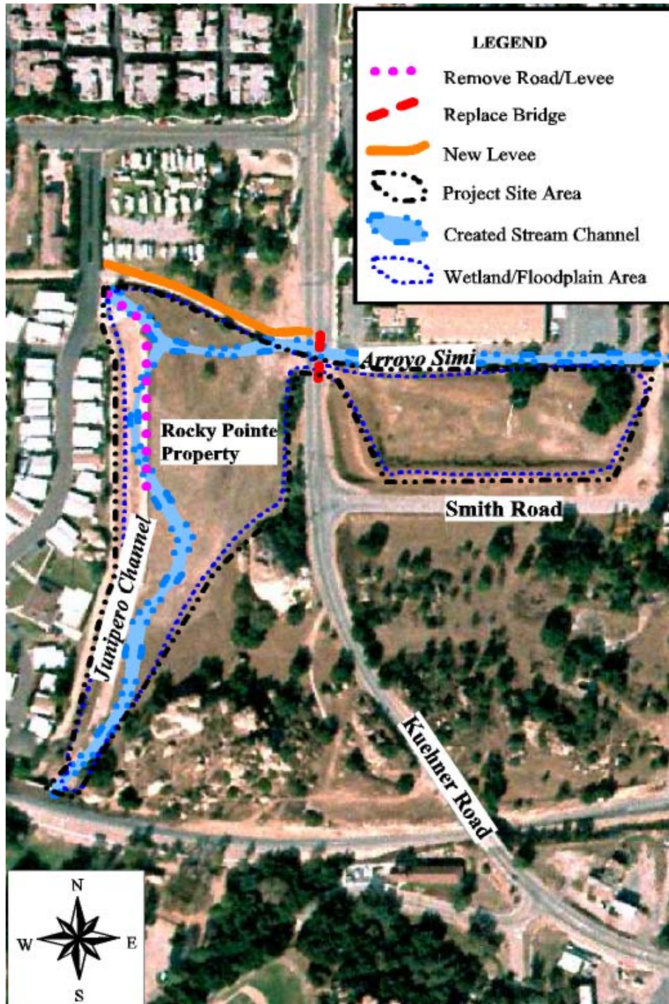
Figure 42. Conceptual Restoration Design for Arroyo Simi/Junipero Channel Confluence at Kuehner Road (Sites 40/41)
